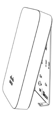
Then adjust the MR30H to guide the MR30H's bottom slot into the cradle's bottom tab until it clicks into place. Once in place, the MR30H should be secured to the cradle by using one of the included screws in the cradle's bottom tab.
