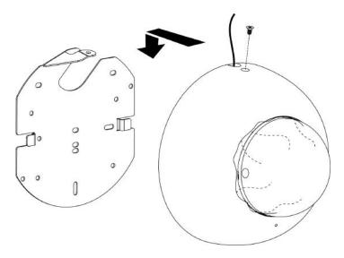
6. Turn bubble counter clockwise to unlock. Hinge bubble off of body to remove.
