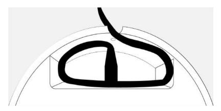
5. Slide camera over top of mount plate and slide down into mount plate hooks. Secure with Phillips or Torx head safety screw.
