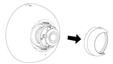
8. Aim the lens. Look through the camera on the Meraki Dashboard to fine tune the picture. The camera sensor and lens unit can be physically tilted through a range of 65 degrees, rotated through a range of 350 degrees, and panned through a range of 350 degrees. The image can only be rotated by 180 degrees in software and no other adjustments can be made. Zoom and focus can be adjusted remotely and can not be adjusted physically on the camera.
