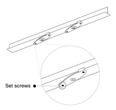
4. Attach the T-rail clips to the T-rail by rotating them and snapping them into place as shown. The black foam pads should be compressed slightly after installation.
