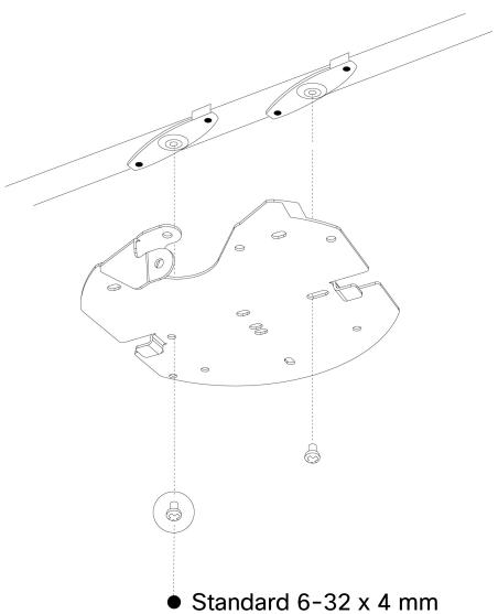
Standard 6-32 x 4 mmT-rail screws
