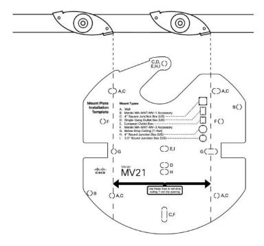
3. Attach the mount plate to the T-rail clips using the mount plate holes (marked with a "G").
