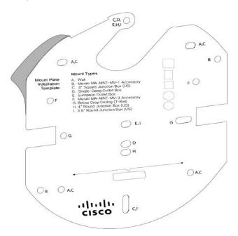
3. Screw the mounting plate onto the wall in pre-determined locations. Use template holes marked with the letter "A" for standard wall mounting.
