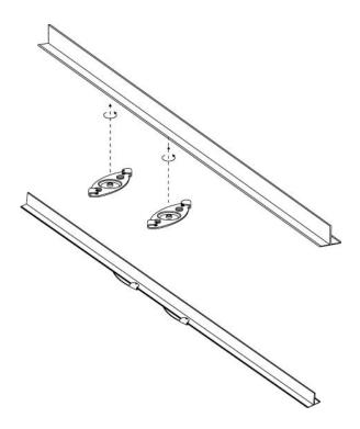
2. Tighten the set screws on the T-rail clips and secure them using a 5/64" (2 mm) hex key.
