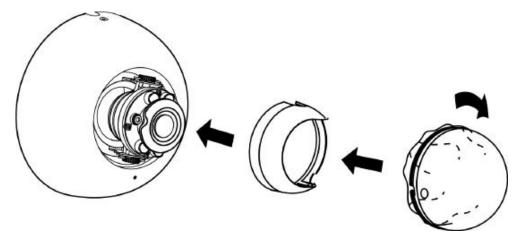
10. Remove protective plastic sticker. Check LED function. Use the Meraki Dashboard to adjust camera focus and configure other settings.
