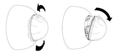
7. Pinch near thumb screws and pull straight away from the camera to remove lens guard.
