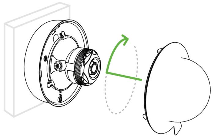
9. Remove protective cap from camera bubble.
