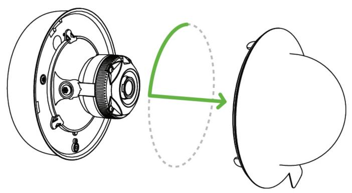
5. Align camera to mounting plate studs. Slide camera onto studs and turn camera clockwise to secure camera to plate. If cable run is not coming from directly behind the camera, the cable guard will need to be removed. Below are two mounting examples.
