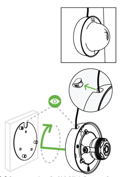
6. Further secure camera to mounting plate by tightening the green security screw.
