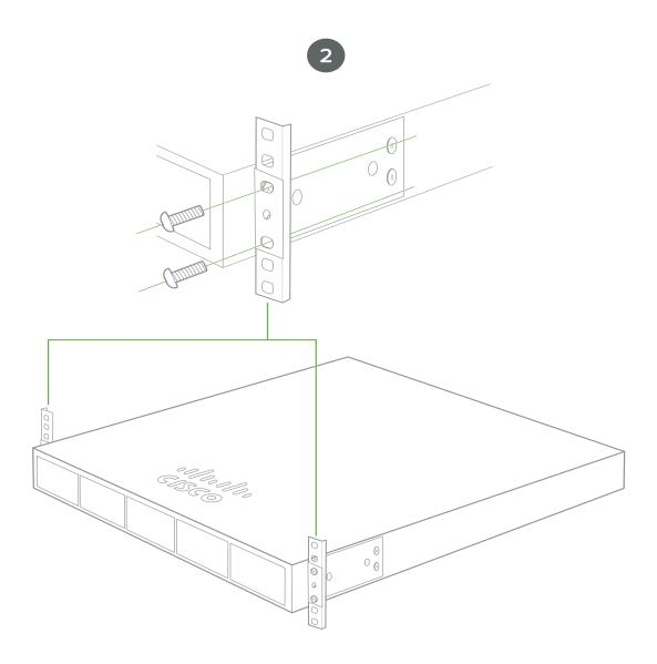
3. Secure and screw in the rack mount bracket on to the rack.
