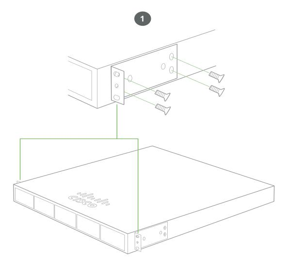
2. Align the rack mount brackets on the sides of the switch onto the rack.
