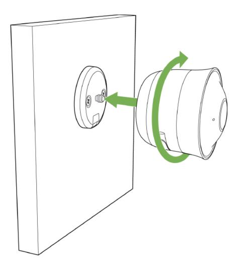
The notch on the mount should line up with USB-C slot on the camera after its mounted
